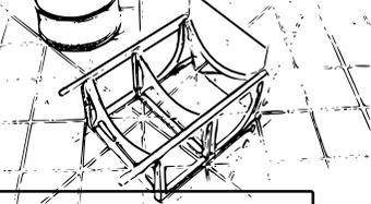
7. From the thick card, carefully separate the framework for one barrel. Parts 1-5.
