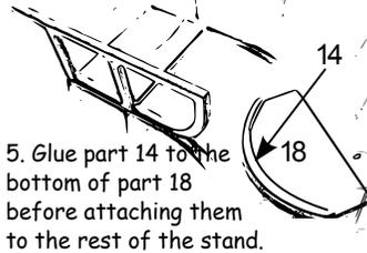
5. Glue part 14 to the bottom of part 18 before attaching them to the rest of the stand.
